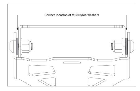
FASTEN (M10) LOCK-NUTS SNUGLY BUT ALLOWING ROTATION OF MOUNT.
