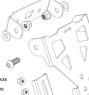
FIT TWO (M8 X 16) CARRIAGE BOLTS IN SQUARE HOLES FROM FRONT OF UPPER MOUNT THROUGH SLOT IN LOWER MOUNT. FASTEN (M8) LOCK NUTS LOOSELY TO ALLOW ADJUSTMENT LATER.
