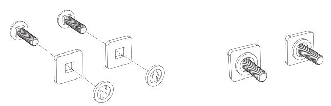
ASSEMBLE TWO (M8 X 30) CARRIAGE BOLTS THROUGH RAIL NUTS AND NYLON RETAINER WASHERS.
