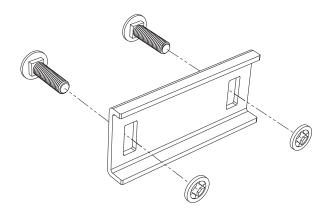
ASSEMBLE TWO (M8 X 30) CARRIAGE BOLTS THROUGH SLOTS IN FLANGE CLAMPS TO NYLON RETAINER WASHERS.
