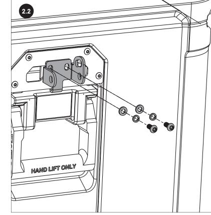
KEEP CLAMP VERTICAL AS SHOWN WHILE TIGHTENING SCREWS WITH M4 ALLEN TOOL TO SECURE FIRMLY IN PLACE.
