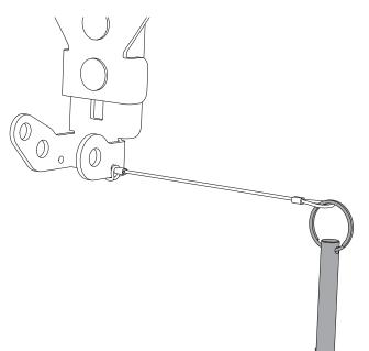
3. ATTACH LOOSE END TO KEY-RING ON QUICK RELEASE PIN. REPEAT FOR OTHER MOUNT.
